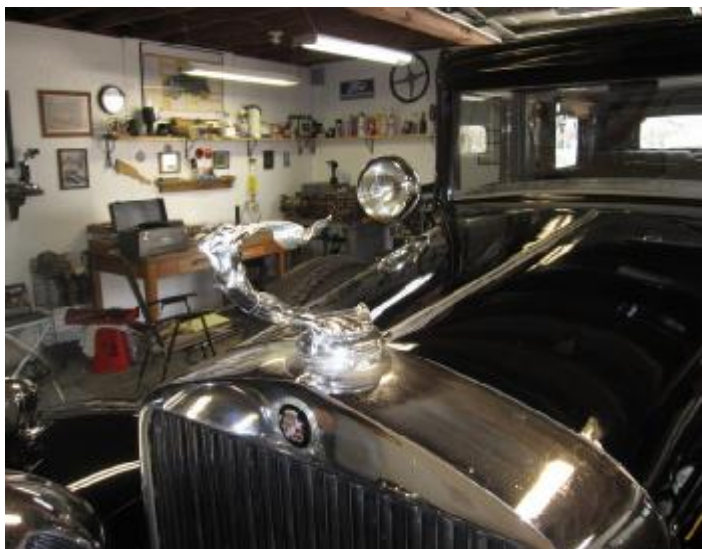
The Radiator louvers are thermostatically controlled, the hood ornament is "The Goddess"
